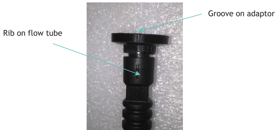
Figure 1.11 Photograph showing the alignment of marking on flow tube and adaptor to ensure component is correctly tightened
